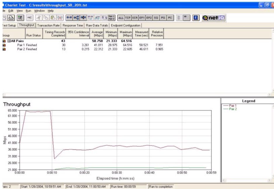
Figure 2-11. Super G Network with 802.11g Introduced Into the Environment at 20 Foot Distance In Open Air
