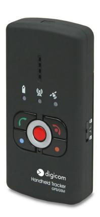
It is equipped with the **GeoFence function** that allows to set restricted geographic areas so that Personal Tracker will send warning messages whenever the monitored object crosses the zone (in or out).
