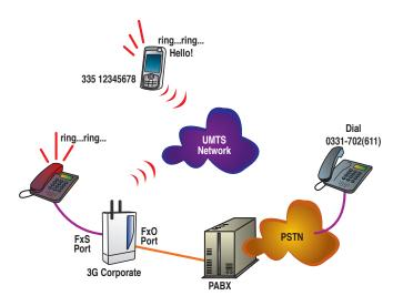
The voice applications of 3G Corporate allow its use as sole gateway in the most performing PABXs where the Internet connectivity is often required to take advantage of all the VoIP functions and Systems Messaging.
