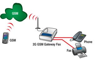
2G GSM Gateway Fax QB can be easily connected to the PABX and become the second line.
