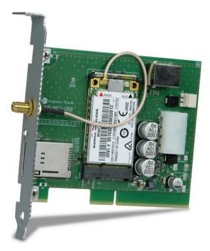
Digicom 3G Modem USB Internal has been projected as a traditional internal device for personal computer (modem, audio cards, etc). This allows to insert it into a PCI SLOT (used for the mechanic mounting only).
