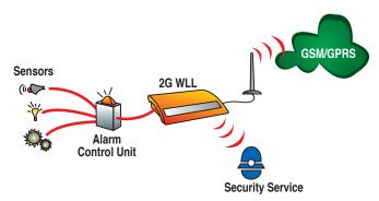
wihout any additional configuration, the phone calls will be made through the GSM network.
