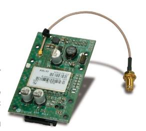
2G Bulk is a Quad-Band GSM /GPRS modem (850/900-1800/1900 MHz) designed to be integrated into professional equipments and to be used for Data (CSD & GPRS) and SMS applications.
