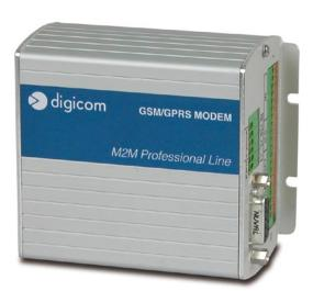
You can also remote interact by sending appropriate SMS that will pilot the opening/closing of the 6 outputs.
